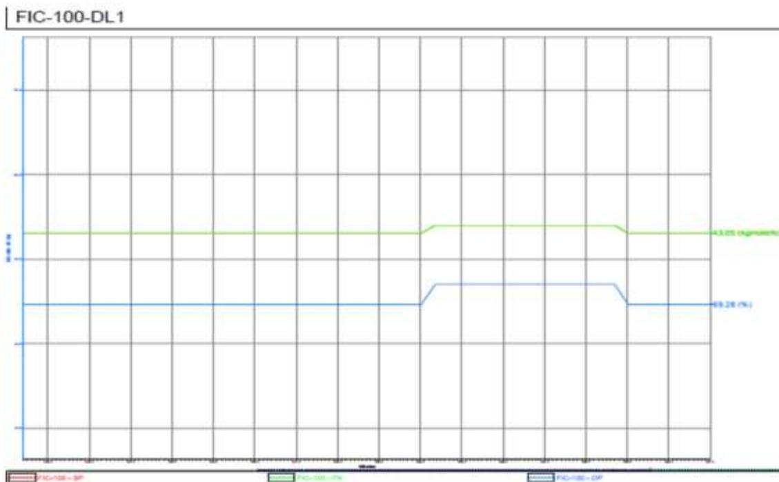
Figure 3 Dynamic response of PI controller FIC-100.
