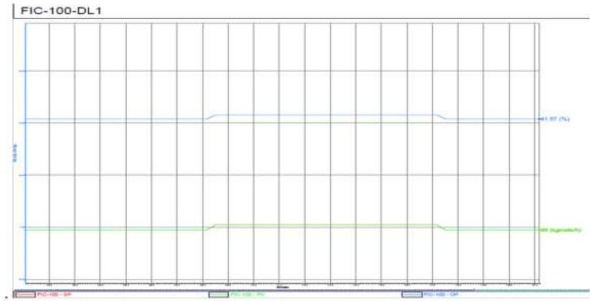
**Figure 3 Dynamic response of PI controlled FIC-100 for PFR-100.**
