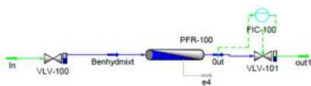
The flow controller controls the product flow rate. Here the product is cyclohexane at a rate of 99 kgmol/h. The first order transfer function with a time constant of some seconds is consistent, which means that first order function may be lag the response of the actuator position changes to the desired actuator position [14]. The controller tuning parameters are decided on using
